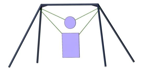
The metal plates for shooting distances up to 300 meters should be made from steel sheets with 16-20 mm thickness, in order for them to be relatively heavy enough, so that they don't roll or turn over, after a hit.
